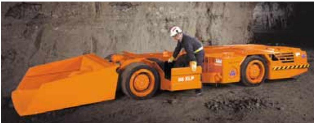
Sandvik Mining and Construction's unique low-profile loader is only 88 centimeters high.
