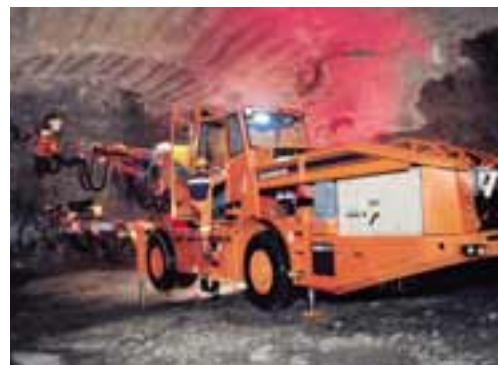
In the underground drilling area, expansion of the new generation of drilling rigs for drifting and tunneling in the Axera series continued.
